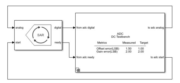
Double click the ADC Testbench block to open the Block Parameters dialog box. Click the **Plot DC analysis results** button to view the ADC transfer curve, endpoint nonlinearity and best fit nonlinearity.
