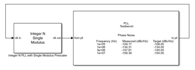
Double-click the PLL Testbench block to open the Block Parameters dialog box. Click the **Plot phase noise profile** button. The PLL operating frequency is 2.8 GHz, and the measured phase noise profile matches the target profile.
